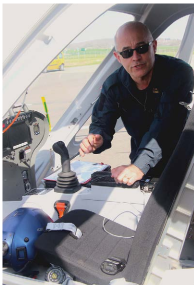
Volocopter test pilot Paul Stone discussing the cockpit of the company's X2 demonstrator during acoustic signature testing at Pontoise Aerodrome, France, in 2022. The control inputs are made through the single stick.
