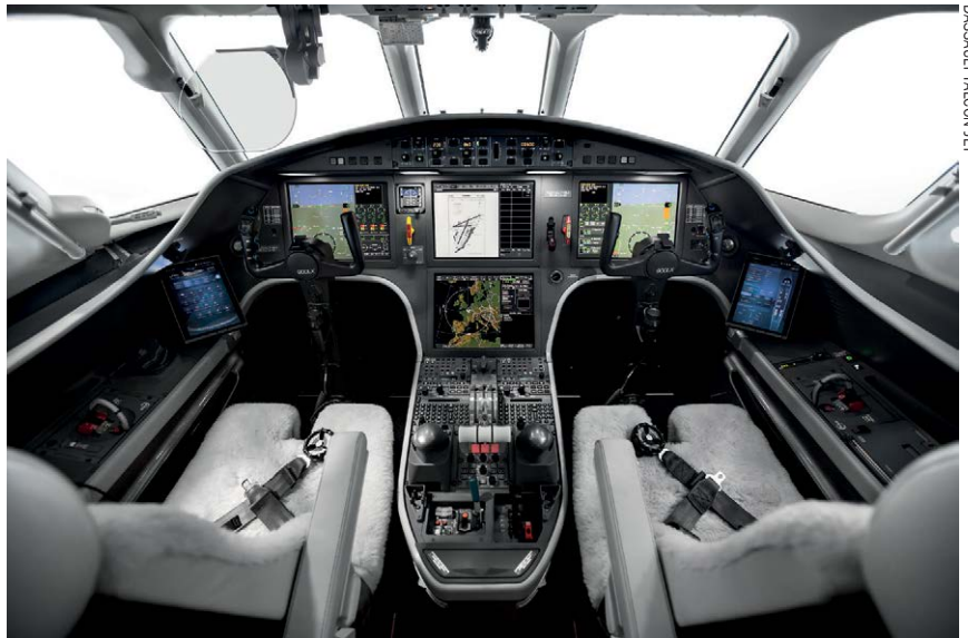
The Honeywell-based EASy II flight deck of the current-production Falcon 900LX.
