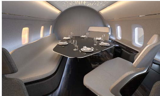
F/List Shapeshifter concepts use bio-based materials with pneumatic functions allowing flexibility even for wood-based veneers.
