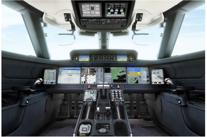
Flight deck features dual Collins Aerospace HGS-6200 HUDs with both synthetic and enhanced vision.
