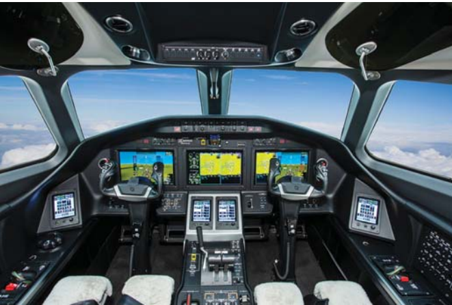
The cockpit features Garmin G500 touch-screen avionics. The optional Garmin HUD and Elbit EVS are slated for 2020 approval.
