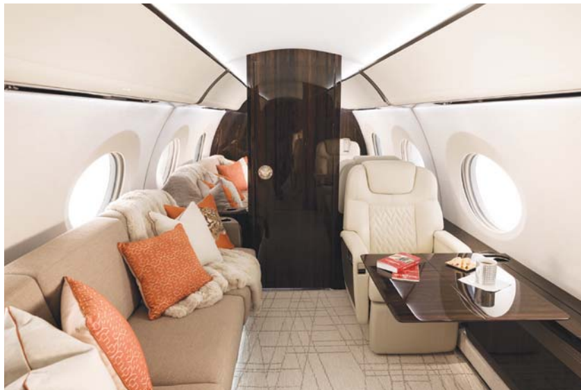
The G600 is 7-in. wider than the G550 with 7-in. more leg room in each cabin section, plus 16% larger signature wide oval cabin windows also used in the G650. The aft private stateroom has a fold-out sofa sleeper and a pair of facing chairs.
