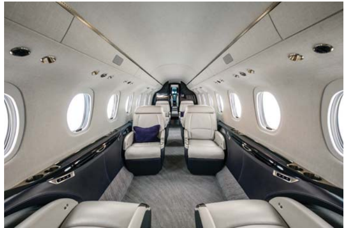
The Longitude's flat-floor cabin has the same lean 6.4 ft. wide by 6.0 ft. tall cross section as Citation Latitude.
