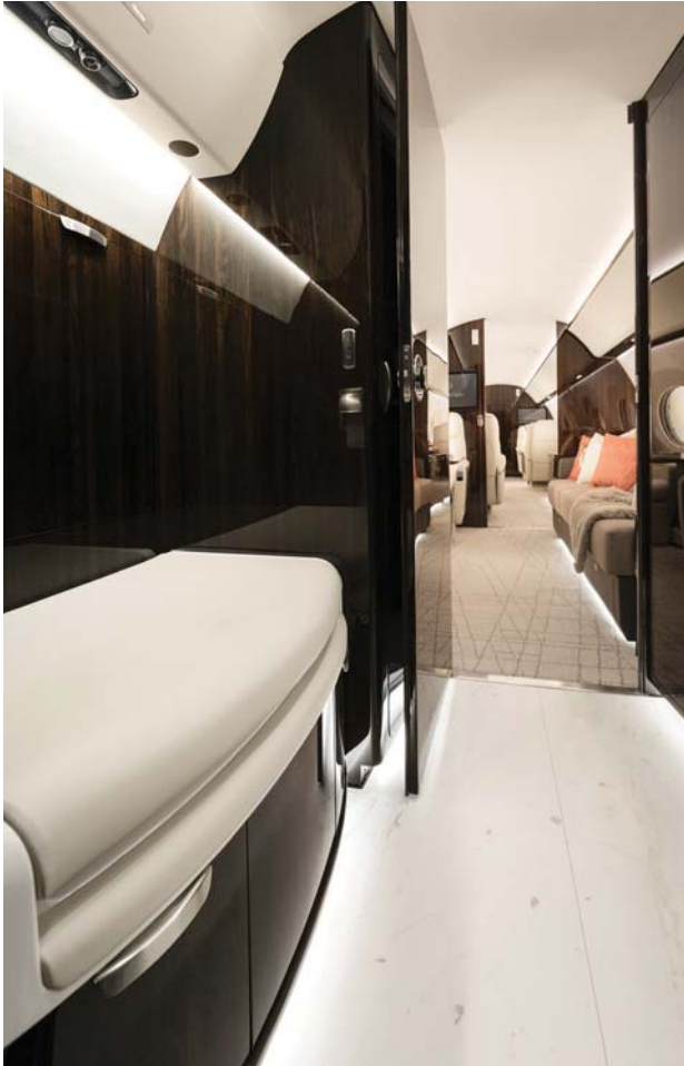
Interior is 3.7-ft. longer than the G500, making room for forward crew rest and larger galley (not shown). High capacity, front and rear vacuum toilets are standard. Chairs are larger and plusher than in the G550. Cabin altitude and sound levels are lowest in this class.
